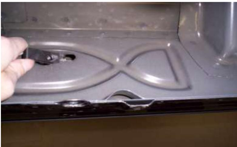
Remove the round plastic cap covering the large hole with a screw driver located on rear of the rocker panel. Slide a spring clip into hole until it snaps into the other hole.
