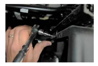
Tip the driver seat back to get access to the under side of seat, on 2011 & newer 4 door wrangler you will have to remove the bracket holding the OEM electrical plug by removing the two Torx 30 screws. Snap the electrical plug from bracket by pressing the clip on under side of bracket with a pair of pliers.
