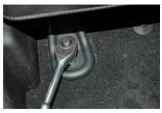
Slide drivers seat forward to access the rear seat bolts. Remove the bolts with a 18mm socket on ratchet.
