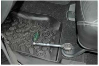
Slide drivers seat back to access the front seat bolts. Remove the bolts with a 18mm socket on ratchet.
