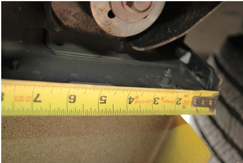
Measure from the front wheel well at lowest point on pinch weld to locate bracket positions.
