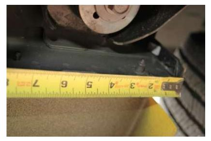
Measure from the front wheel well at lowest point on pinch
