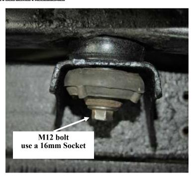
Using a 16mm socket remove the body mount bolt at each of the 3 locations on each side.
