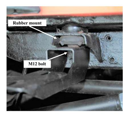
Place the rubber mount onto the vehicle and the bolt through the bracket then through the rubber mount and tighten back into the vehicle all locations.
