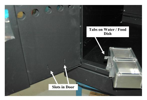
Place the water / food dish tabs into the slots in the door and slide down to secure onto the door.
