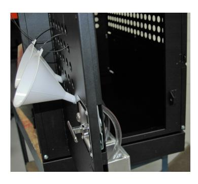
Slide the hose onto the funnels, then slide hose through the bottom outer holes in door routing the hose into each of the compartments in water / food dish. Secure to the door with cable ties as
