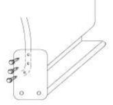
Level board and attach stone guard to vehicle using the sheet metal screws that are included or drill holes in the stone guard in the locations of the screws removed from the OEM plastic stone guard.
