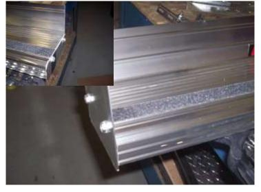
Attach the stone guard and end caps to the board with 3/8" self threading bolts. (extruded board shown)
