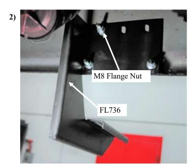
Place the FL736 bracket onto the stud coming out from the back of the rocker panel, for each location.
