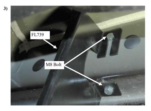
Attach brackets to vehicle by inserting a M8 x 20 mm bolt into each of the threaded holes in back of rocker. Tighten bottom bolt first then the top bolt. For each bracket location.
