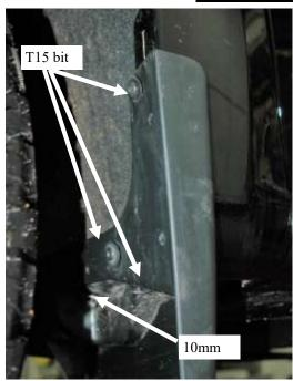
Remove the small factory stone guard in the front fender well by removing the small screw with T15 and 10mm socket and then unsnap. Keep screws to reinstall the screws.
