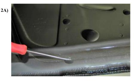
Remove the round plastic cap covering the holes with a screw driver located on rear of the rocker panel. This exposes the M8 threads in vehicle to mount bracket.
