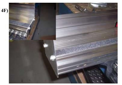
Attach the stone guard and end caps to the board with 3/8" self threading bolts. (extruded board shown)
