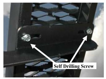
Place the board on the brackets and center on the cab of the vehicle from front to rear. Attach to the brackets using #14 X 3/4" long self drilling screws.
