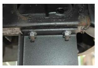
2) Place the FL503P bracket up onto the threads of the stud plate (30-3410) and place two nuts onto the threads and tighten. Repeat to the driver side with the FL503D also.
