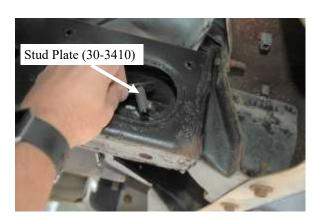
1) Place the stud plate (30-3410) through the oval cutout in rear frame rail. Insert the threads down through the holes in lower flange of the frame rail. **Repeat to the driver side also.**
